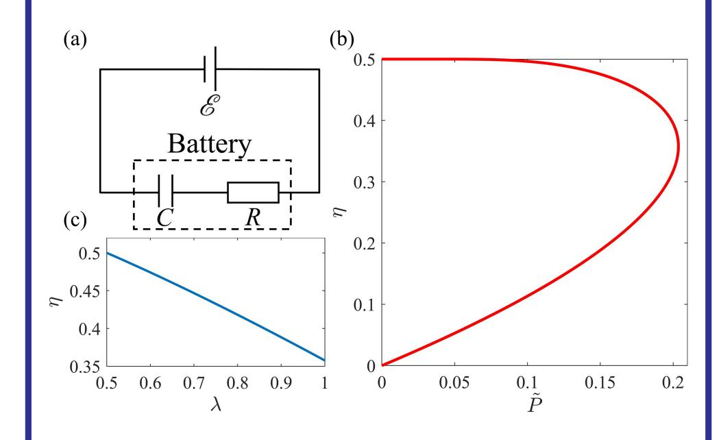
For the simplest RC circuit, the voltage and charging current of the battery are
