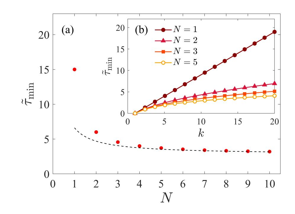
In the regime of  $N \gg 1$ , retain the first order of  $N^{-1}$  of  $\tau_{\min}$  as  $\tau_{\min} \simeq CR \ln k + CR \frac{\ln^2 k}{2N}$ , indicating 1/N-scaling of decay.
